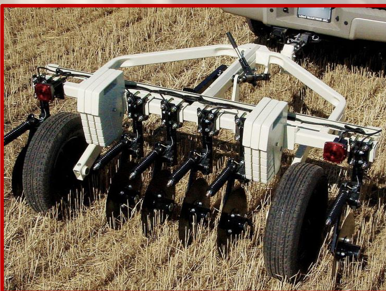
Figure 2 An example of a Veris soil EC collector
