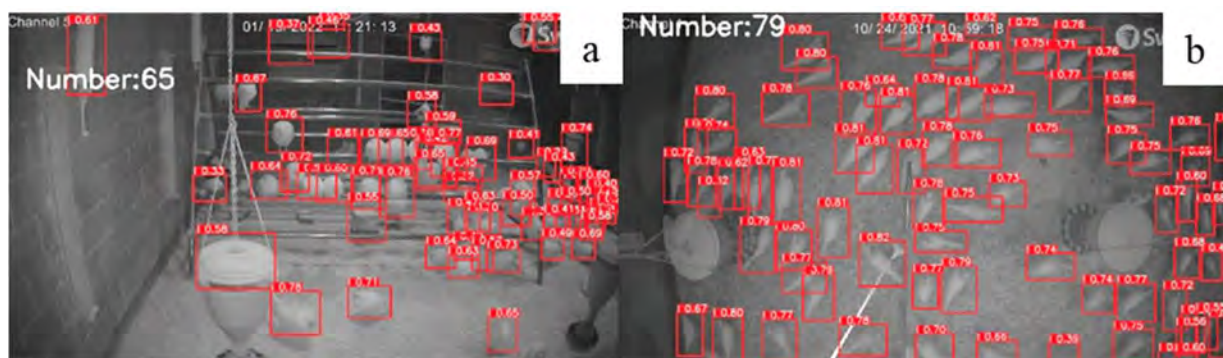
Figure 1. Number of chickens identified at different angles by a machine vision system: horizontal angle (a) and vertical angle (b).
