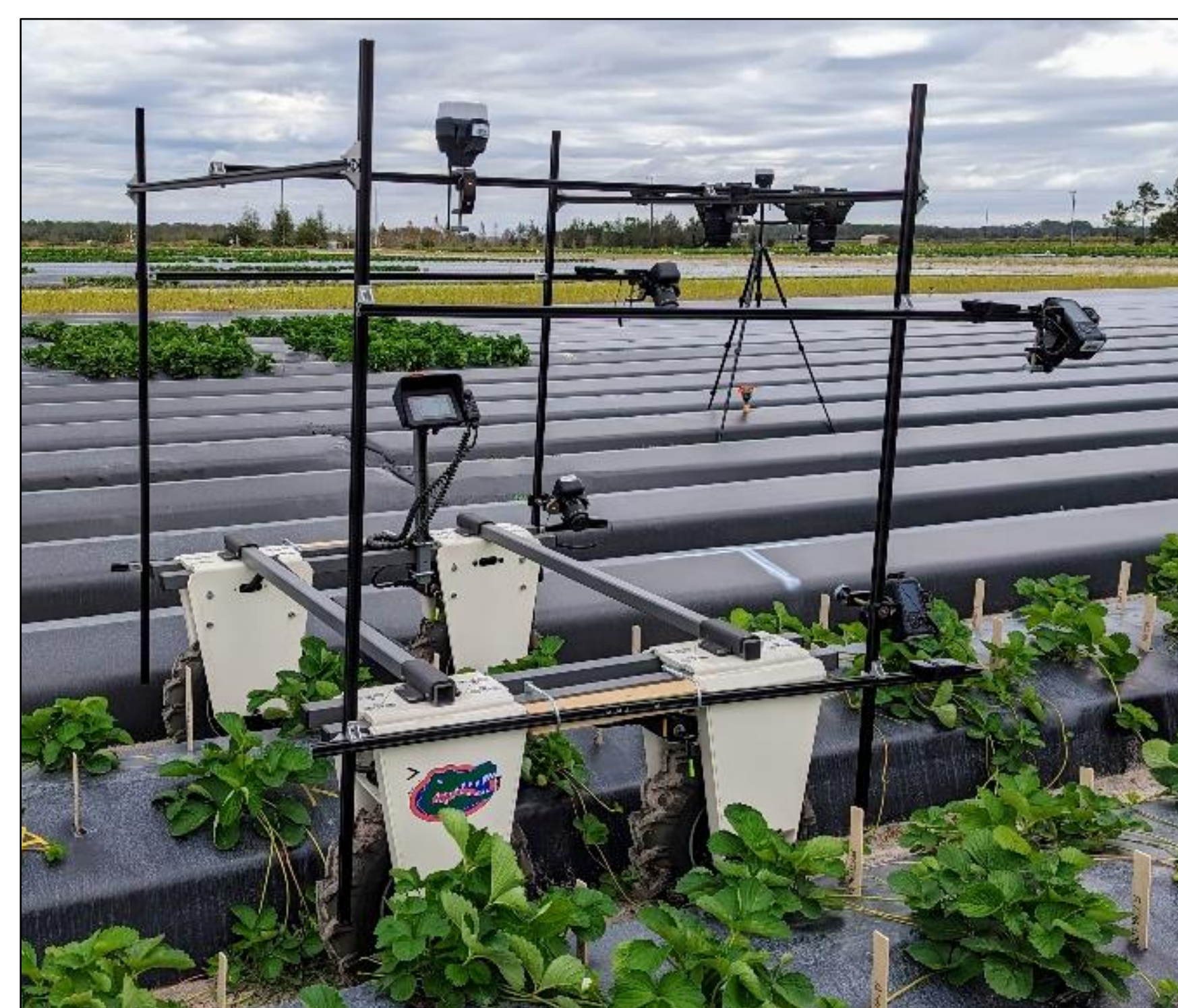
Figure 2. A ground imaging system for strawberry phenotyping
