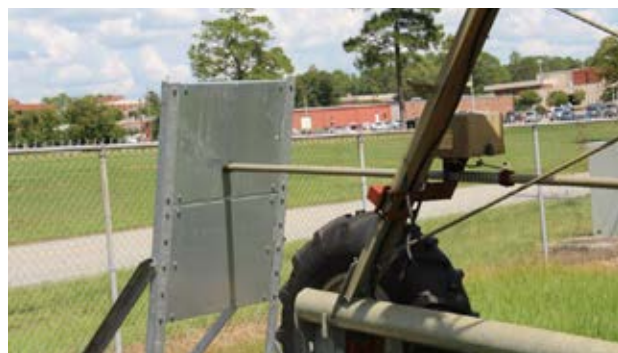
Figure 13. The stop and safety switch on a pivot. In this case, if either switch malfunctioned, the pivot would walk over the fence and into the road—a very dangerous situation.
