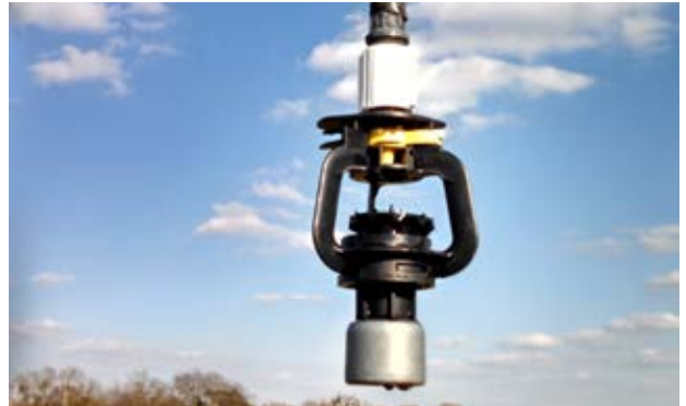
Figure 7. A new sprinkler on a drop hose. There are visible differences between new and older/worn sprinklers, which affect both appearance and operation.
