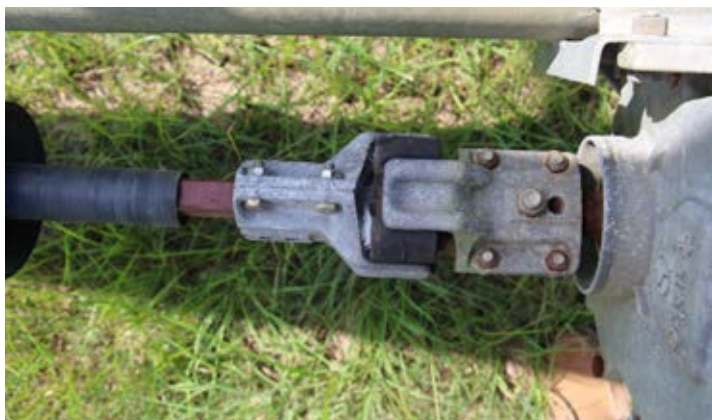
Figure 17. Close-up view of the universal joint and driveline connection point. Rodents and insects love to inhabit these areas, so use caution when opening and inspecting. Clear, clean, and replace parts as necessary.
