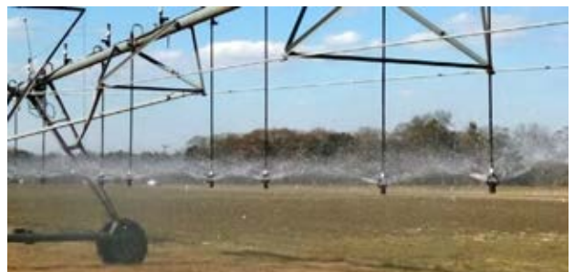
Figure 9. Nozzles operating on a center pivot system. In some instances, uniformity or other nozzle-related issues can be observed through visual assessment. Sprinkler uniformity can be quantified using the methods described in UGA Extension Circular 911.
