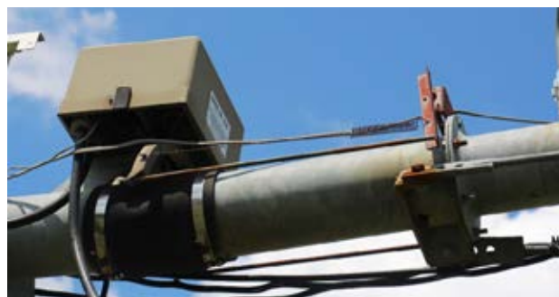
Figure 12. An alignment switch located at the connection point between two pivot towers. Ensure that all components on the alignment system are in working order. Replace any components that appear worn and may not last through the season.
