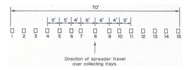
**Figure 1.** A field layout of collection pans showing extra clearance on each side of the center pan for spreader wheels. All pans are placed at 5-ft intervals except for pans 7 and 9, which are placed 6 ft from the center pan (No. 8).
