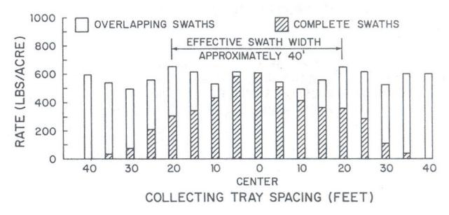
**Figure 2.** The spread pattern is determined by collecting the material in trays/pans and pouring it into test tubes. Material overlap, as shown, results when swath spacing equals the effective swath width. This is a typical pattern one might expect from a dual spinner-disc fertilizer spreader. This does not depict an ideal pattern.
