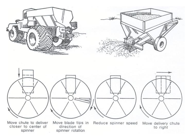
**Figure 5.** Four adjustments to correct heavy right distribution patterns from a single spinner-disc fertilizer applicator. These four corrections allow material to ride the spinner further and deposit toward the left side. Corrections for heavy left patterns are opposite to those shown for heavy right patterns.
