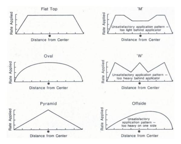
**Figure 3.** Typical dual spinner-disc spreader distribution patterns. The three patterns (flat top, oval, and pyramid) shown on the left are acceptable while the patterns (M, W, and offside) shown on the right are not desirable and need spreader adjustments to generate an acceptable pattern.
