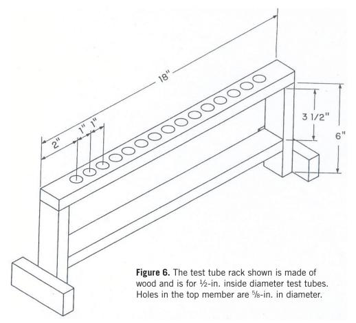
Calibration kits (including collection pans, tape measure or rope marked at pre-determined intervals, test tubes, and test tube rack) are also available for purchase from various fertilizer application equipment manufacturers or dealers at a reasonable cost.
